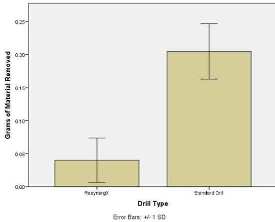
Figure 3: The standard drill bit captured, and removed from the site, more than 4 times the amount of material (combination of bone marrow and cancellous bone.) than the Self Grafting drill bit which removed less than 0.05 g from the bone tunnel created (fatty material).
